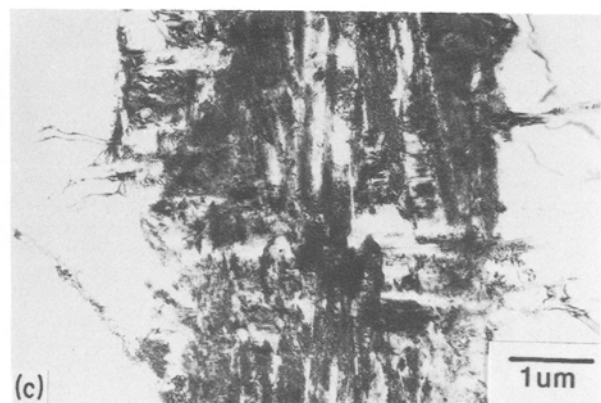
Figure 4 Typical microstructures of samples heated to (a) 1213, (b) 1243 and (c) 1323 K.
